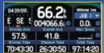
The trip information page displays present speed, distance travelled and other helpful statistics.
